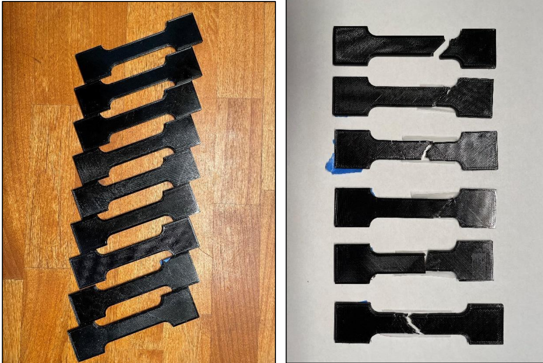
A2: Dog bones before and after testing, in order of testing
